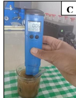
(A) Weighted 5g of soil (B) using glass rod stir the solution. (C) Measure the EC using EC meter.
