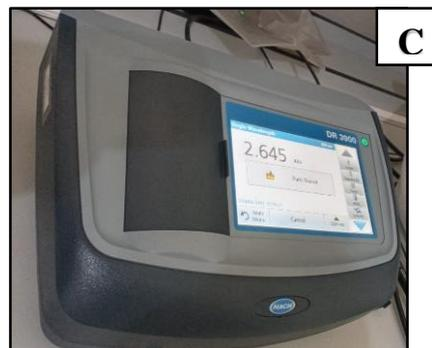
(A) Shake the soil sample using mechanical shaker (B) filter the extract using filter papers (C) get reading using spectrophotometer.
