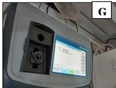
(A) soil sample shaking using mechanical shaker (B) solution added into centrifuge tube (C) the tube was put in the centrifuge machine (D) prepare the sample for get spectrophotometer reading (E) after adding reagent into the sample (F) put the prepare sample into spectrophotometer (G) get reading in sample using spectrophotometer.
