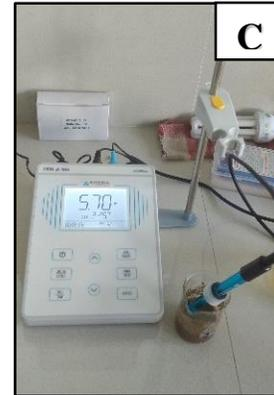
(A) Weighted 5g of soil (B) using glass rod stir the solution. (C) Measure the pH using pH meter.
